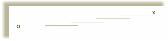
Layout D : Drawing panels to open from Left to Right stacking to the front
