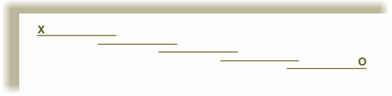
Layout A : Drawing panels to open from Right to Left stacking to the front
