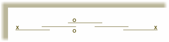
Layout E : Drawing panels to open from Center to the Left and Right stacking to the back
